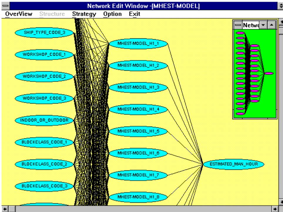
Figure 12. Neural Network Configuration for Manhour Estimation
