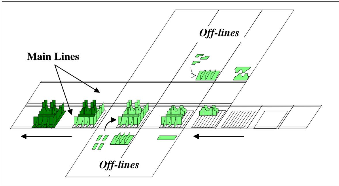
Figure 10. The Panelled Block Assembly Shop with Assembly Line and Off-lines.
