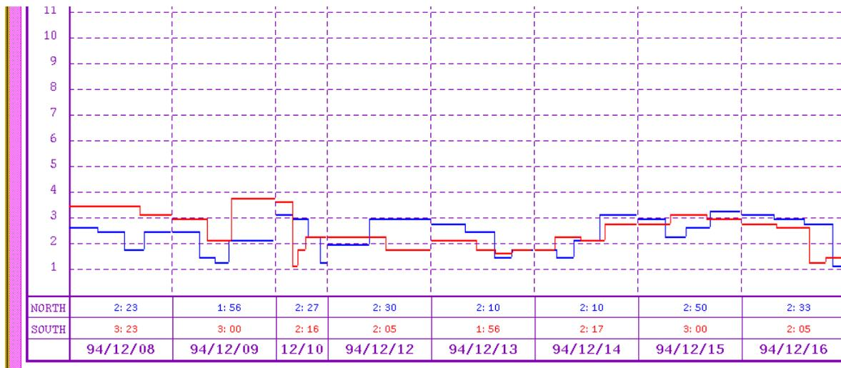
Figure 11. Output Screen Showing Dynamically Changing Cycle Time in DAS-PANEL
