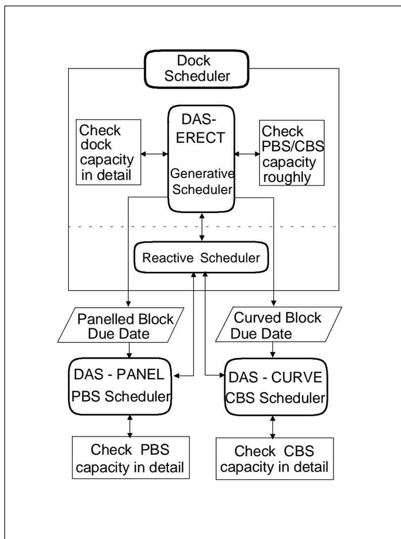
Figure 3. Hierarchical Architecture of Shipbuilding Scheduling.
