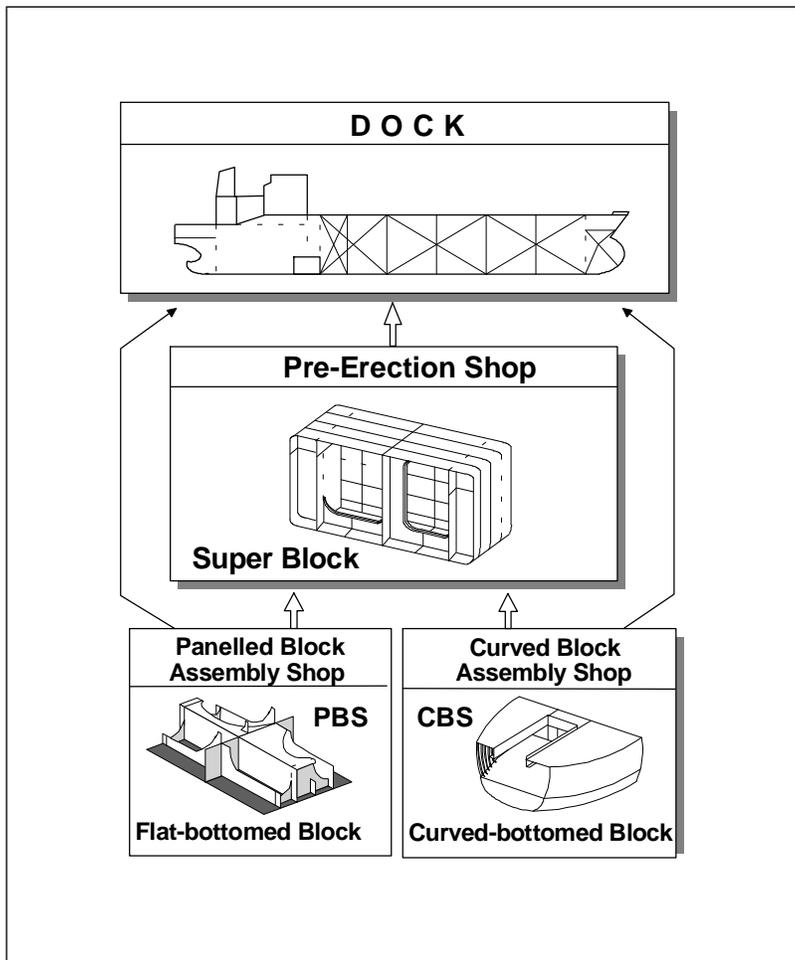
Figure 2. Typical Shipbuilding Procedure.
